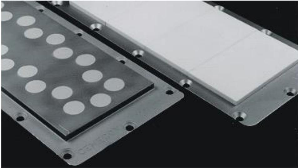
**Fig 8:** Titanaluminum (left) and alumina (right) soldered on copper plate
