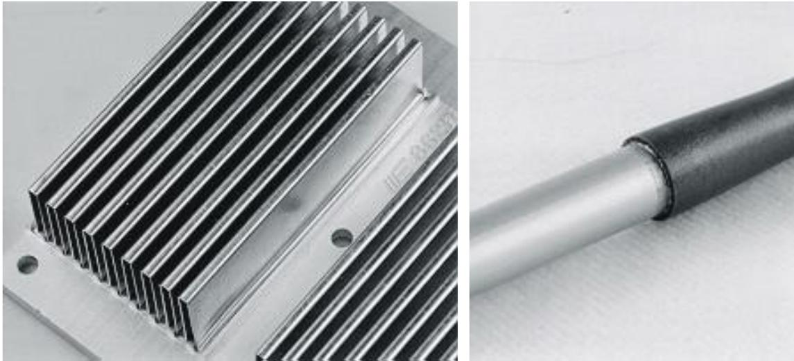
**Fig. 6:** Fins (AlMgSi0,5) - solder # 1 – plate (AlMg3) (left) and tubes (Al and Cu) (right)
