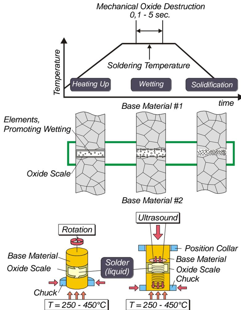
**Fig. 1:** Soldering principle with mechanical oxide removal and methods of oxide destruction
