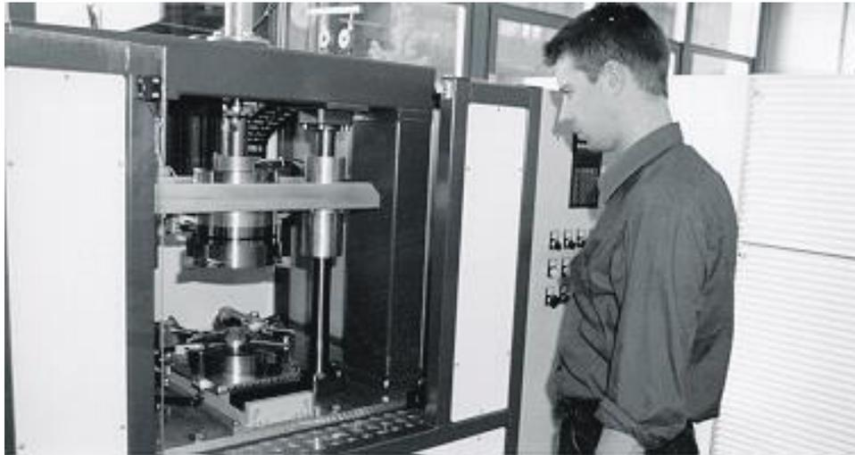
**Fig. 3:** Special installation for fluxless soldering operation
