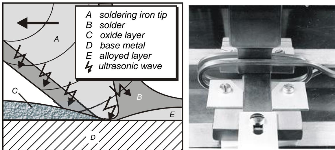
**Fig. 2:** Ultrasonic soldering iron (left) and induction coil with horn (right)
